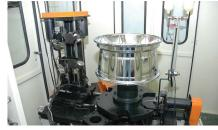
Tire radial force and wheel radial run-out first harmonic play a significant role in the ride quality of a vehicle. Matching and mounting tires on wheels is a process wherein a tire's position on the wheel is specifically selected to help minimize the effects of the final combination force variation and / or imbalance.
